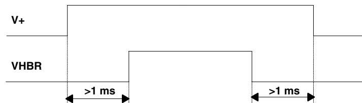
Figure 3–1. Recommended Power-Up and Power-Down Sequence
